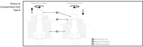
Remove the side panel on the temperature control unit to loosen and tighten the transportation locks.
