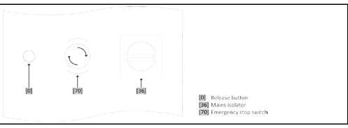
**INFORMATION** By activating the **>Emergency stop switch<** [70], all poles of the temperature control unit are disconnected **immediately**.
